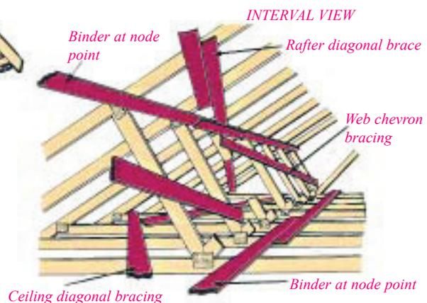
(One only shown and spliced) webs and all other bracing omitted for clarity. Braces to be 25 x 100mm free of all major defects and fixed with two 3.35 x 65mm galvanised nails at all cross-overs including wall plate. Braces to be inclined at approximately 45( to the tiling battens and repeat continuously along the roof.
