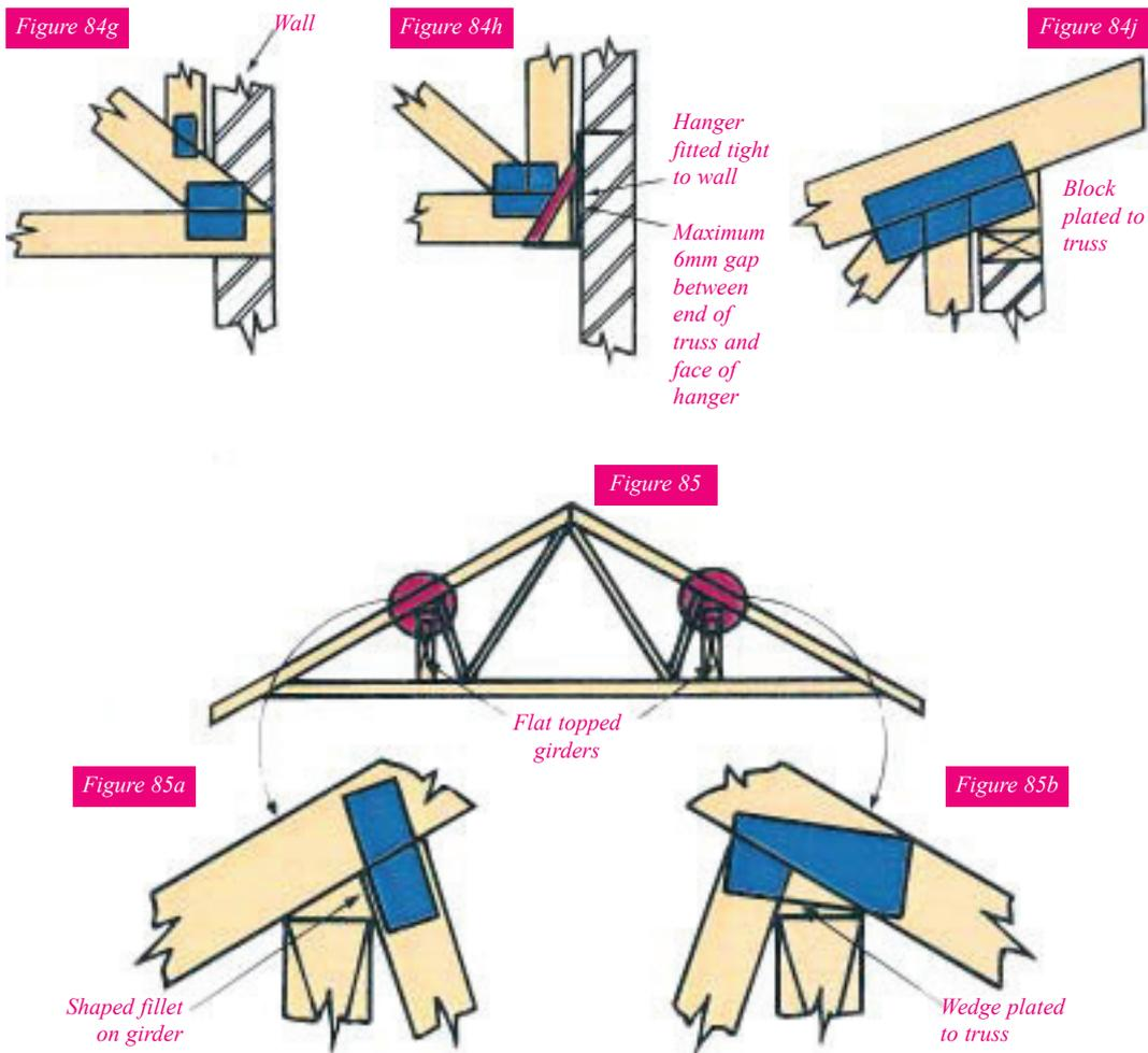
Top hung fixings (figure 84j) are not common since, at ceiling level, the wall generally needs lateral restraint from the roof against wind and the ceiling ties need to be stabilised.
