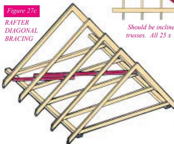
Should be inclined at approximately 45( and each nailed to at least three trusses. All 25 x 100mm free of major defects and fixed with 3.35 x 65mm galvanised nails at all cross-overs.
