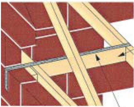
Noggings to be provided and set horizontal unless the strap has a twist to line it up with the roof slope
