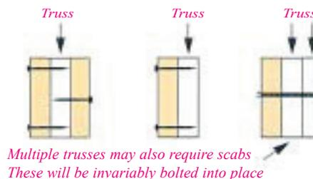
Nails and bolts should either be inherently corrosion resistant or protected by a corrosion resistant coating.
