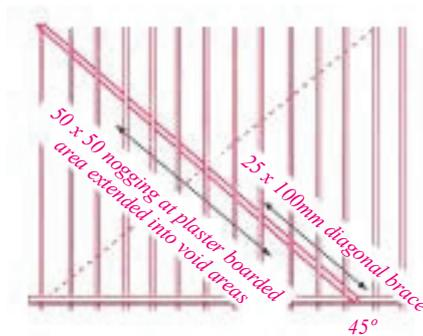
Note: Bracing shown must be installed both sides of ridge and repeat at intervals (with a minimum of two) along roof. Alternate rising to left and to right. Where the roof is short the second line of bracing may cross as shown by the broken line.
