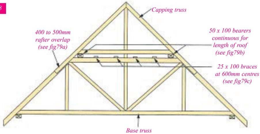
The two tier truss (figure 78) comprises a flat-topped base truss and a triangular capping truss, fitting alongside the base truss on longitudinal bearers. Each truss may be one of a large selection of types. The base truss will generally be made as high as practical but not so high that the span of the capping truss is less than 2-3m. Although a duo-pitched shape is shown in figure 78, all basic configurations can be constructed by the two tier method.
