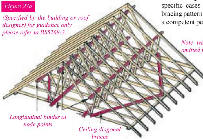
BS.5268-3 gives some recommendations for certain specific cases of roofs; for other types of roof the bracing pattern for roof stability should be designed by a competent person. See figure 27a, 27b, 27c and 27d.
